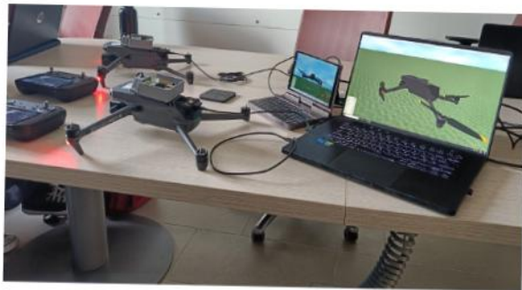
Figure 2: In-hardware simulation of two DJI drones. Two separate instances are running on their own simulation, while the Raspberry boards are still able to share messages.
