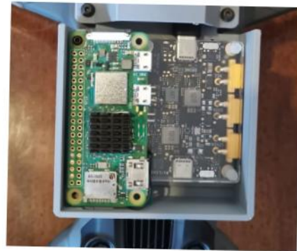
Figure 1: The complete payload mounted on top of the Mavic 3E, with both the E-Port Development Kit, and the Raspberry Pi Zero 2W.
